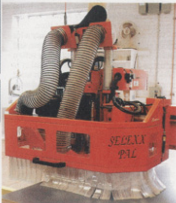
THIS COMPUTER-ASSISTED MACHINE MAKES PRECISE CUTS, PRE-DRILLED HOLES AND ROUTINGS AT YANKEE REMODELER.
