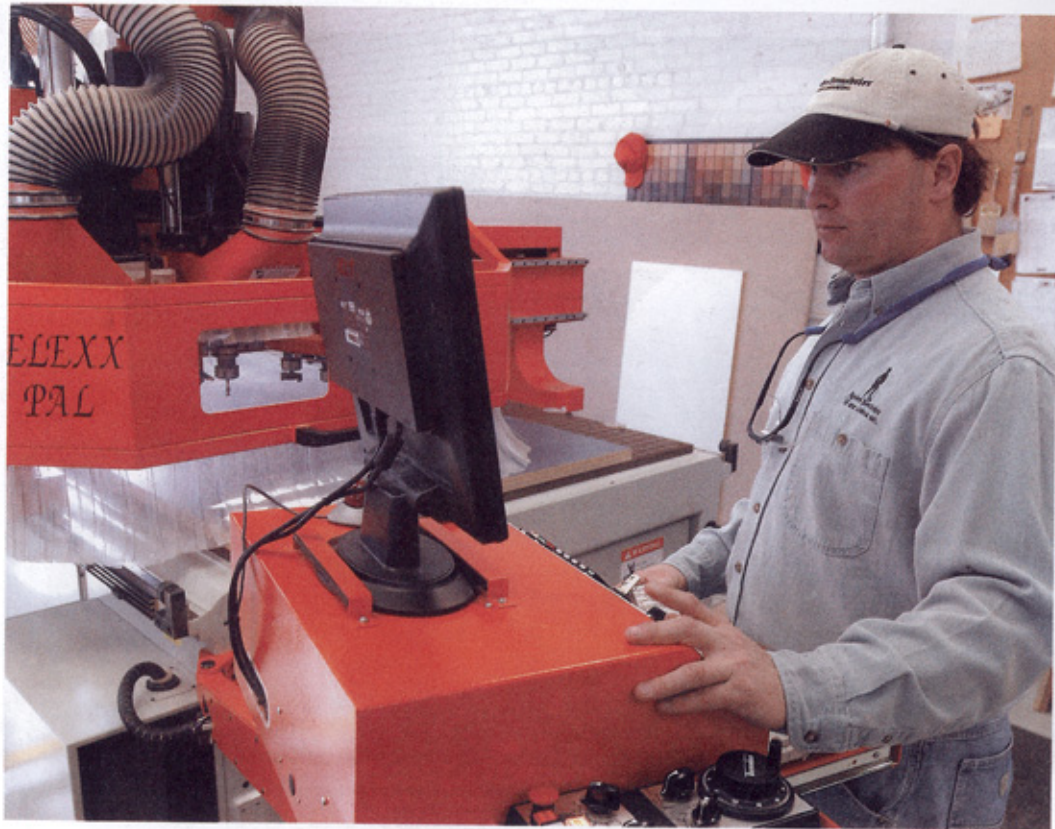
MIKE MAHONEY, SHOP SUPERVISOR AT YANKEE REMODELER OF NEW LONDON, GETS THE NEW OMNITECH SELEX COMPUTER-CONTROLLED ROUTER READY TO RUN. THE COMPUTER-ASSISTED MACHINE TAKES A CUSTOM DESIGN FOR CABINETS OR SHELVES AND MAKES ALL OF THE PRECISE CUTS, PRE-DRILLED HOLES AND ROUTINGS NEEDED FOR THE PRODUCT. JEFF EVANS PHOTO
